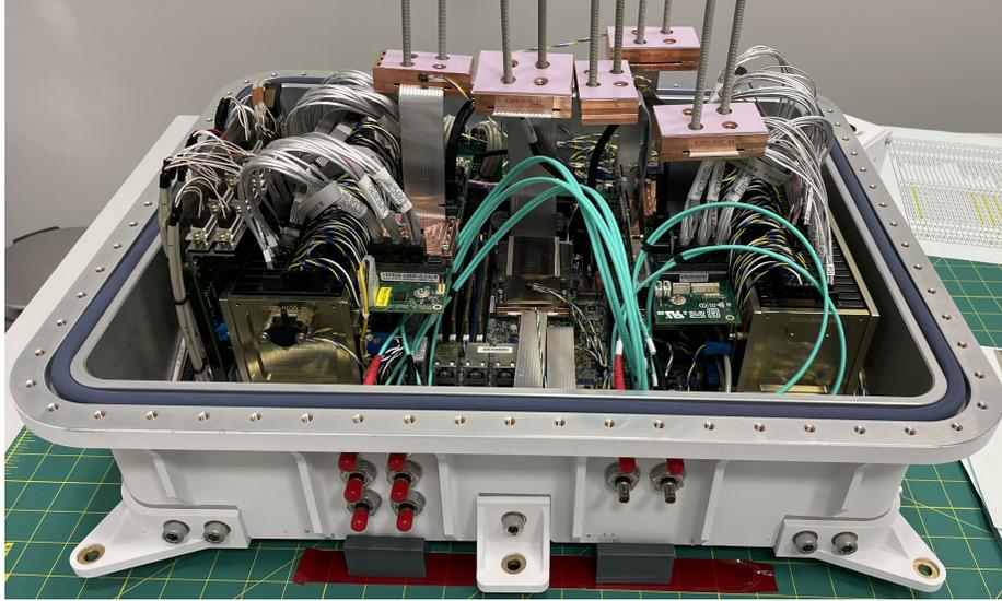
**Figure 20.** ICS shortly before the final closing in October 2021. The mainboard of the ICU is at the bottom of the housing, left and right are the two DSS stacks containing the SSD disks. Identified hot spots on the electronic boards are connected via heat pipes to copper blocks. During the closing procedure, the guiding threading rods are replaced by screws that attach the copper blocks to the lid via gap pads.
